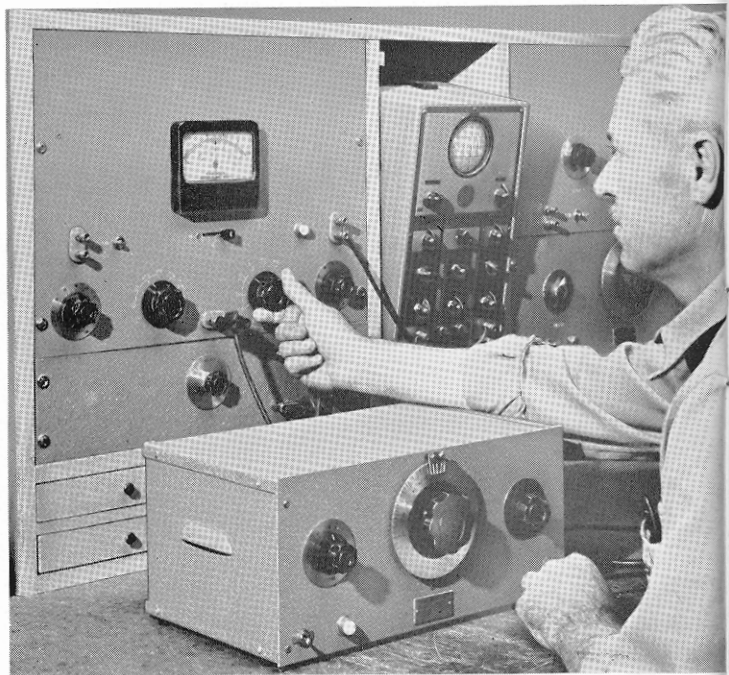
The 325B Distortion Analyzer is being used to measure the total harmonic distortion of a Model 200B on the production test bench.
