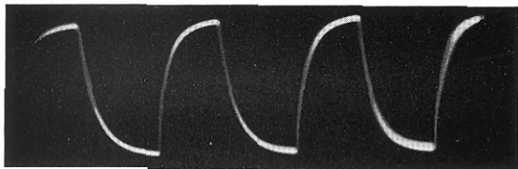
Square Wave Distortion from poor high frequency response.
