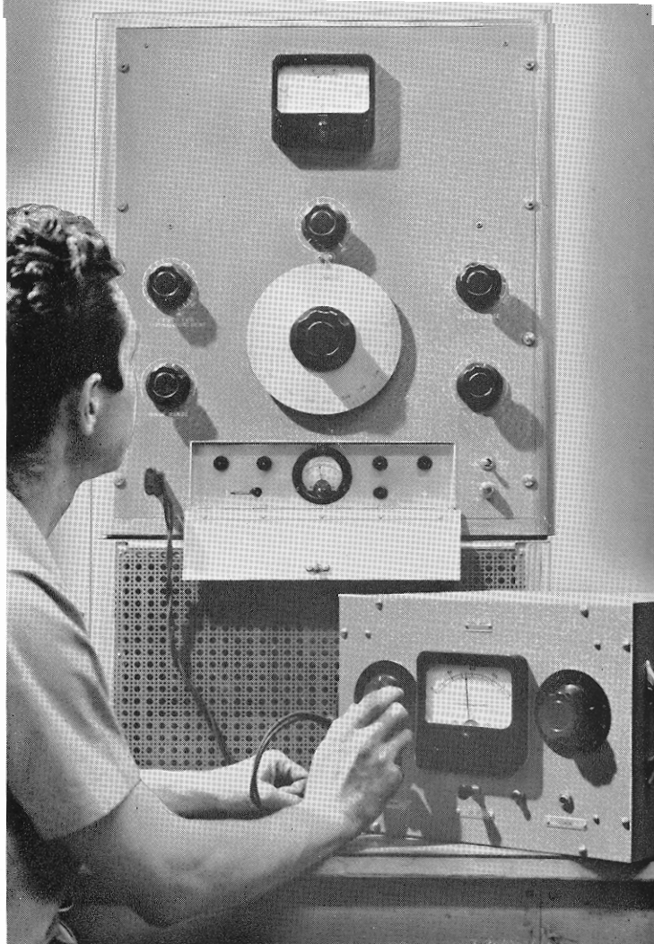
Model 300A Wave Analyzer being used to measure the individual harmonics present in the output voltage of an amplifier.
